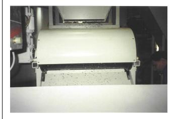
The broken and centrifuged chipping become evenly distributed by an upstreamed vibration gullie and a fast running conveyor transports the chipping to the magnetic field of a rotating magnetic roller equipped with strong permanent magnets.
