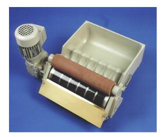
Magnetic separators with a capacity between 60 l/min and 400 l/min have an aluminium cast casing. Machines with a capacity between 400 l/min and 600 I/min welded are constructions made of stainless steel. The magnetic filter system MA 100 (100 l/min for a viscosity of 6 mm<sup>2</sup>/s) can be seen on the photo above. The casing of the magnetic roller has been removed to show the arrangement of the permanent magnets.
