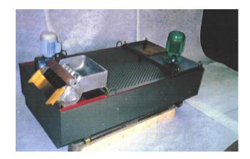
Magnetic separators are also often used as main-filter in a filter system. Our photo shows the filter system FA - MA100 with tank and pump.
